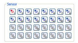
When it sensorsed, relevant sensor icon comes to Red, and indicates sensor number of video.
