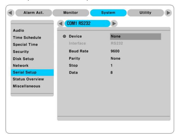
Set connectable device in RS232 in Serial Setup menu to Keyboard. Also set Baud Rate, Parity, Stop, Data with relevant value.
