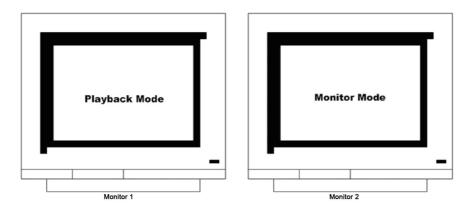
Monitor 1, 2 can search/playback every images in Single or multi divisions. Namely, Monitoring and Playback is possible simultaneously.
