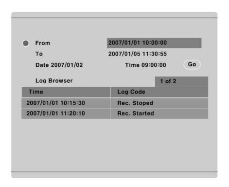
From for the time to start recorded data, To indicates the last time. Select From/To and press [ENTER] to move to the relevant time.
