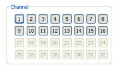
Above picture refer to Off channel 1. In case of Channel Off, relevant button is projected. And video does not come and changed to black screen.
