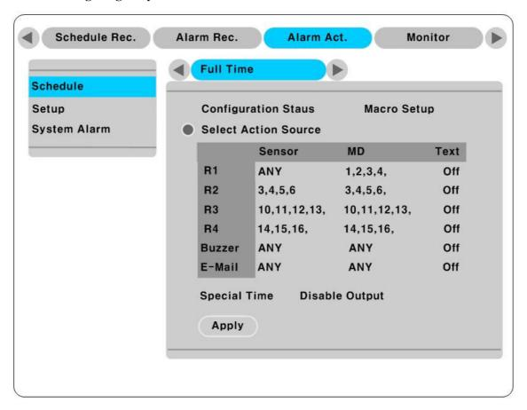
Relay can run by sensor or MD and its condition can be set differently according to schedule. When using the [Relay] button + [Number] button on the front panel or Control Center Lite-D S/W, relay can be operated from remote site.
