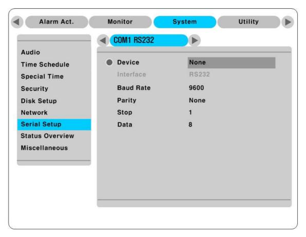
After completing serial setup, configure base address or port for each channel at "Camera menu" tab. When connecting PTZ devices to several cameras, be sure base address matches address for the camera.
