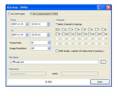
When select avi file format, File Split Size item disappears and replaced to Frame Rate setup and Image Resolution setup item. Also it shows window the select that can includes Audio & Caption.
