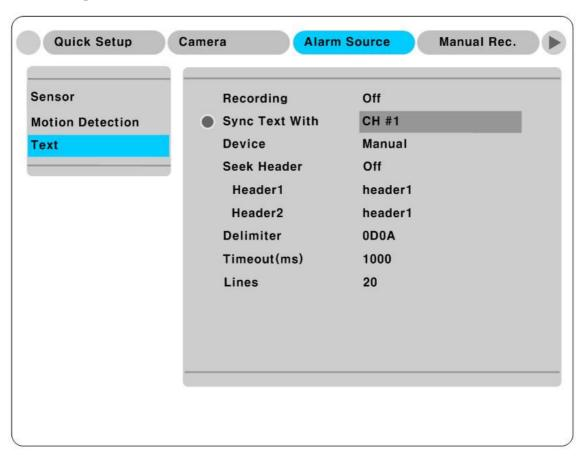
Set Recording & Monitoring menu to all 'On' and set Sync channel to the wanted value. If connectable devuce is Star Finger 007, set the relevant device only. And et other products to Manual and set all inferior menus.
