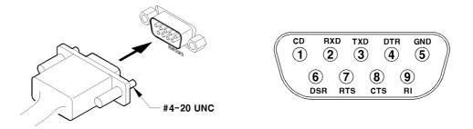
Connect to COM1/RS232 (9Pin D-Sub) of HVRM and configure the "Serial Setup" sub-menu under the "System" tab and "Text" sub-menu under the "Alarm Source" tab shown as above figure.
