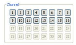
It is On/Off button for the Channel located to left in page. Click the channel wanted to On or Off. And Default is On.
