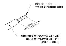
Standard Wire: Peel off the wiring, cover 8~10mm and solder it. Wire gage should be AWG 22~26.
