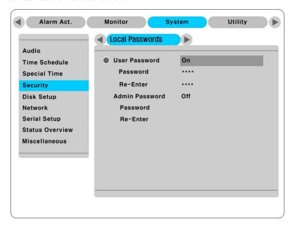
Press [EXIT/LOCK] button over 3 sec. to operate Lock mode with message "Screen Locked" on the bottom of screen. When "User Password" is Off, the message "Enable user password first" is on the screen.
