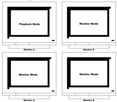
Monitor 1~4 are capable of searching several video/playback in single & divided sreen. Namely, several channels can be monitored and playback separately and simultaneously. But Playback can be monitored in 1 monitor among Monitor 1~4, and the rest 3 monitors for monitoring.
