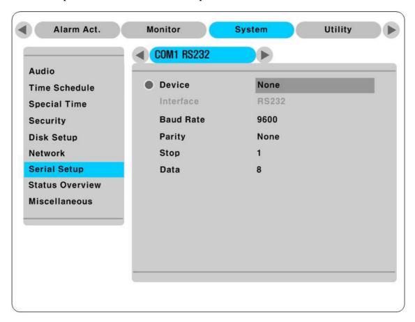
Set connectable device in COM1 of Serial Setup menu, and also set Baud Rate, Parity, Stop, Data with relevant value.
