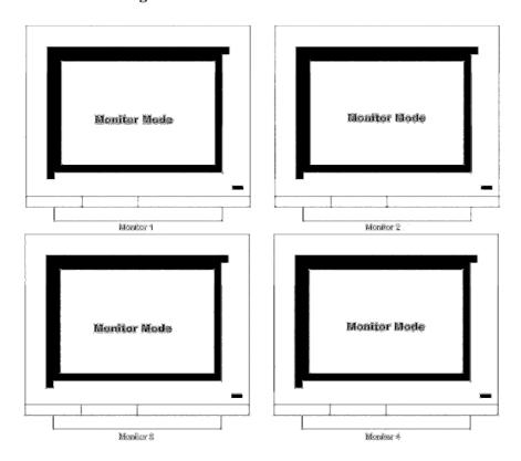
Monitor 1 monitors several video channels, and Monitor 2 is for bigger screen of channel 1. Also Monitor 3 for Sequence mode and Monitor 4 is capable of monitoring Alarm Pop-up images. Every Monitor 1~4 can be set in following conditions separately.
