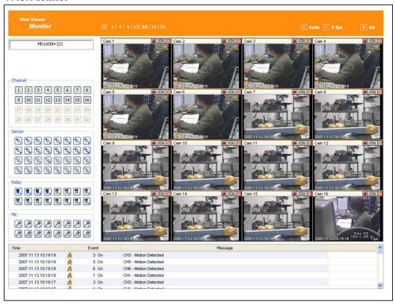
When it is authorized with User ID & Password input at Login page, it moves to Monitor page. At Monitor page, monitor real time image of cameras connected to DVR, or it can control PTZ camera, Relay, and use Microphone function according to user's authorization.
