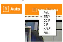
As above picture, click the menu for the menu of resolution. And select out of Auto, TINIY, QCIF, CIF, HALF, FULL, and then relevant resolution is applied to all channels.
