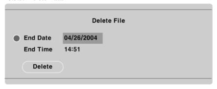
The menu to delete specific rage of data in present HDD recorded. Delected data is limited to present HDD used, and it does not affect to backup disk.
